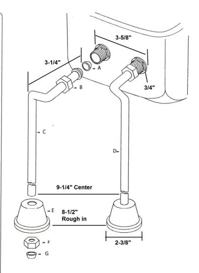
Note:1/2" Compression stops can be used. :3/4" Bevelled washers also provide to use in place of part A if required.
